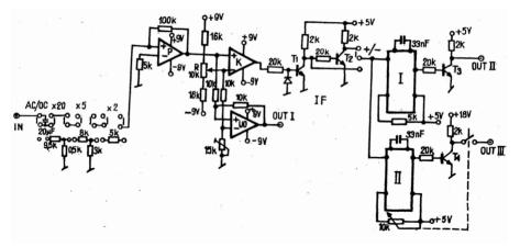
Fig. 1. Schematic diagram of the amplitude discriminator. For detailed description see text.
