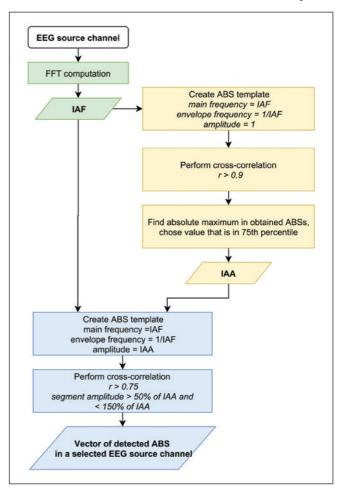
Fig. 1. Workflow of the ABS detection algorithm. The computation step searching for individual alpha frequency is marked with green, the assessment of individual alpha amplitude with yellow and the final computation part with blue.
